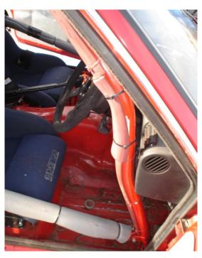
Other issues raised are the mounting feet, the requirements for which are clearly set out within K and the attachment of side bars to main and front hoops. The Regulations provide for such to be welded or bolted. If bolted reference needs to be made to K1.3.7 which details the acceptable designs, looking closely at the photo above you will see a side bar connection that doesn't appear to comply with any acceptable design.
