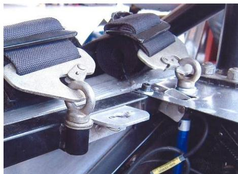
In addition to the issue of the quality of the welding there is an important point in that the after-market mounts protrude significantly above the top surface of the chassis tube, probably by 10 - 15 mm. The effect of this is that through leverage the stress applied is increased.
